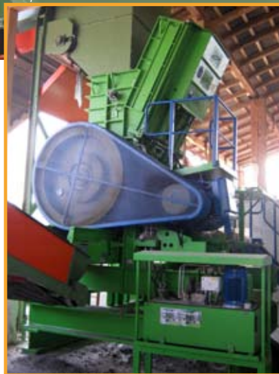
The MeWa UG 1608 MSL Granulator produces substitute fuels.
